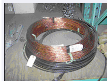
Copper wire containing insulation is often transported to burn sites where the insulation is burned off in a steel drum leaving behind just the copper wire.
